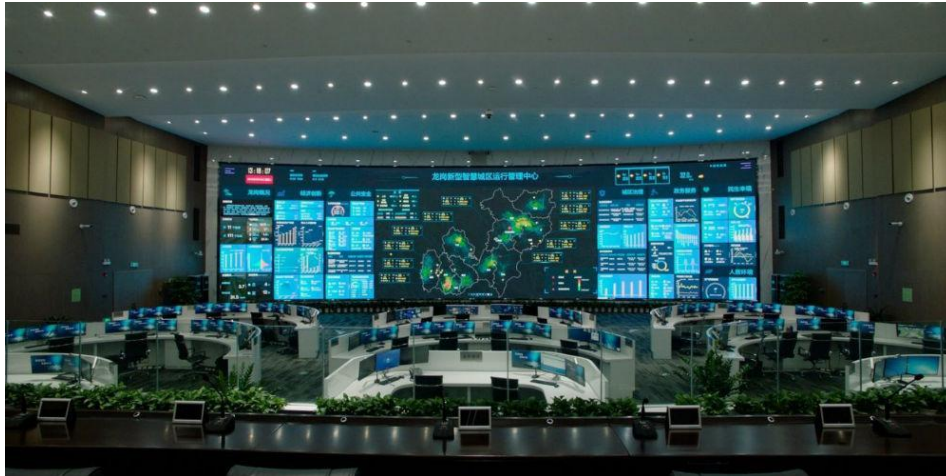
Figure 1. Smart city brain at Longgang Operation Centre (LOC) in Shenzhen: This 166.9 sqm 1.2mm screen is 25.6m by 6.5m and contains a record-breaking 103 million pixels.
